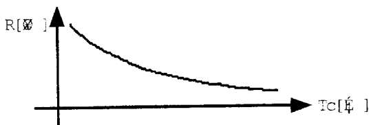
* Temperature and resistance graph for NTC
