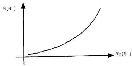
[ Temperature and resistance characteristics of PTC degauss ]
